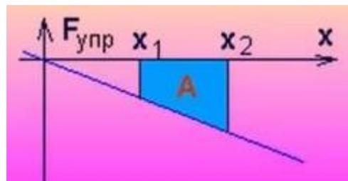
$$A = \frac{F_1 + F_2}{2} (x_2 - x_1) = -k \frac{x_1 + x_2}{2} (x_2 - x_1) = -\left( \frac{kx_2^2}{2} - \frac{kx_1^2}{2} \right) \quad (6).$$
