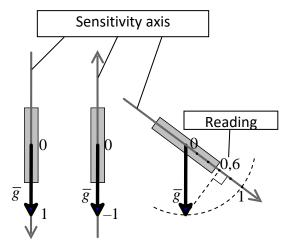
Level 1. Single-channel accelerometer
