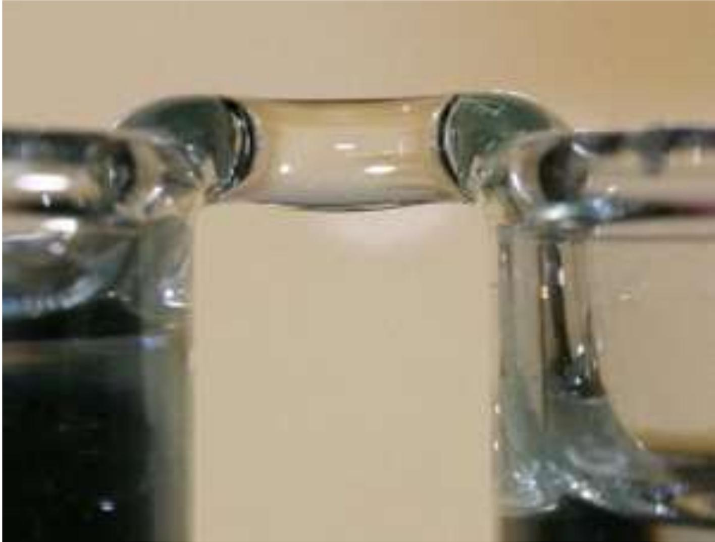
Water forms floating 'bridge' when exposed to high voltage
